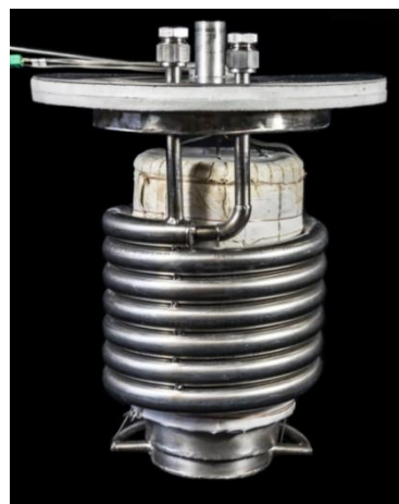
Reactor with heat exchanger and integrated heat supply
