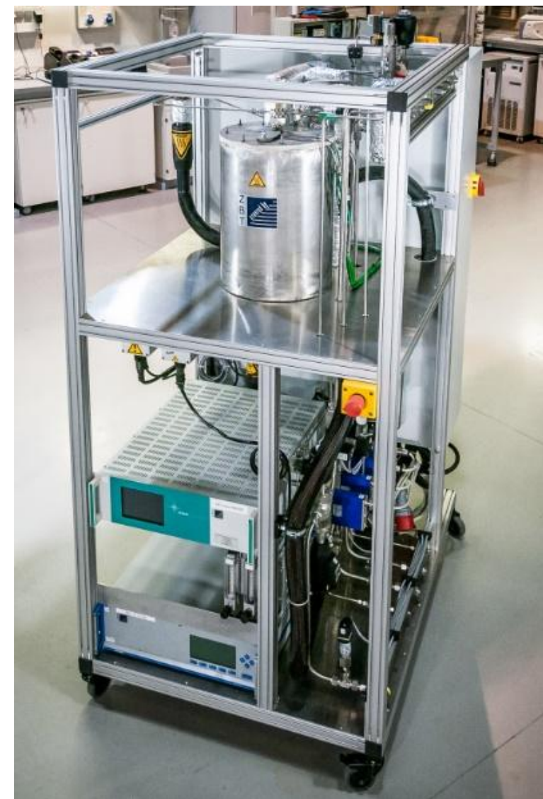
Ammonia cracking plant
