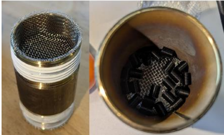
Reactor with catalyst pellets sandwiched between two shaped pieces of mesh
